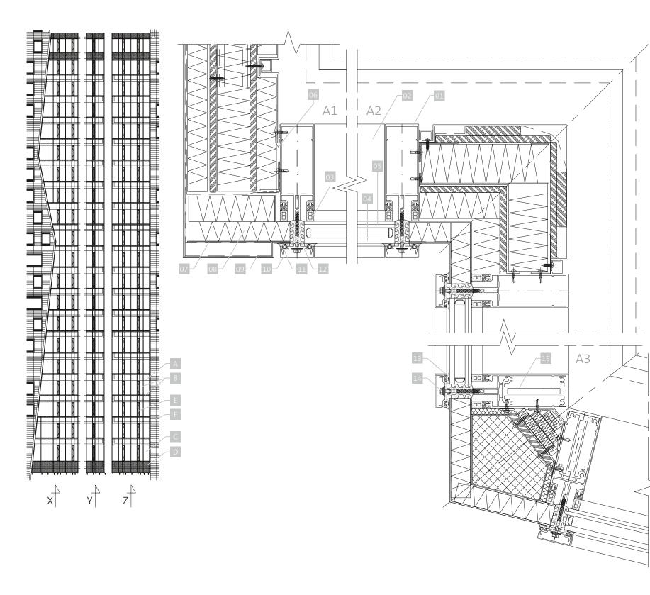
A Building construction - slabsB Stick curtain walling
